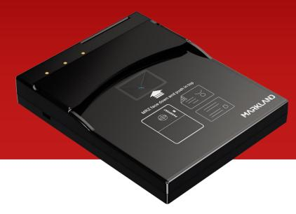
Half-Page e-Passport Reader, Scans MRZ, reading of barcodes, RFID and SmartCard chips
